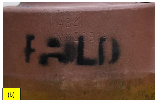
Photograph # 2: As-received condition of the plug valve showing intact external body with red-oxide coating and manufacturer identification markings. No mechanical damage, deformation, or cracks were visible on the outer surface.
